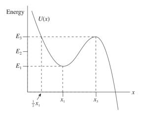
The energies indicated on the vertical axis are evenly spaced; that is,  $E_3 - E_2 = E_2 - E_1$ . The energy  $E_1$  is equal to  $U(x_1)$ , and the energy  $E_3$  is equal to  $U(x_3)$ .
